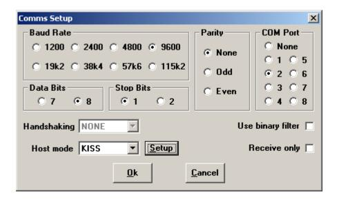
The baud rate selected in the UI-View32 'Comms Setup' screen must match the rate selected for the port in use. Select host mode 'KISS', and be sure to choose the correct COM port for your PC. Click on 'Setup' to continue configuration.
