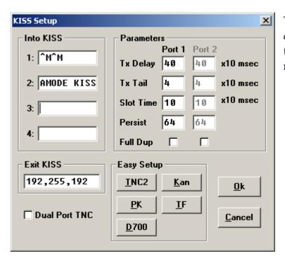
This configuration will only work with port A, as the command console is not available on port B.
