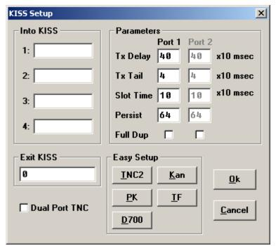
No 'Into KISS' or 'Exit KISS' commands are needed, and any settings in these fields should be deleted. Placing a '0' in the 'Exit KISS' field avoids a bug in UI-View32 that prevents it from exiting properly when the option is left blank.
