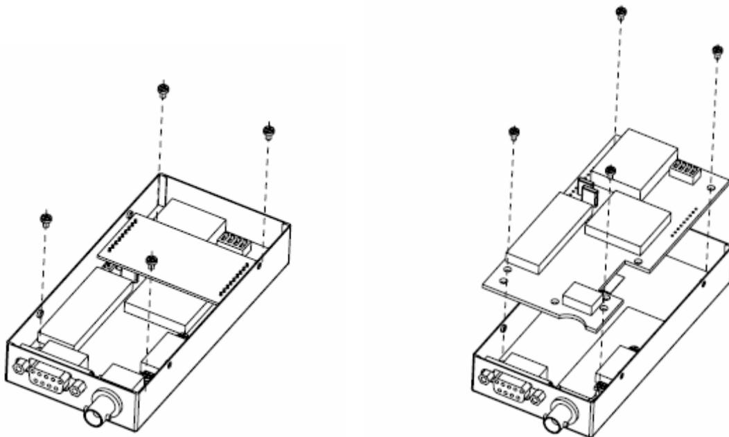
Figure 3 RF BOARD Removal
