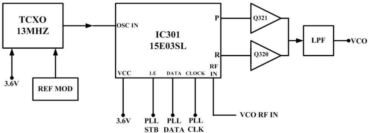
From the above Block Diagram : PLL circuit generates the first local oscillator signal for reception and RF signal for transmission.
