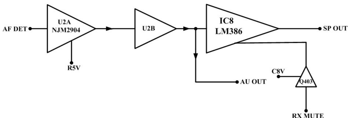
From the above Block Diagram; The resulting AF signal from IC2 enters base band processing chip U2. First coupling by C412 and amplified by U2A ,then it is filtered by U2B which is a low pass filter.After U2B,one signal pass through IC801 and send to COM pin 2, one signal is amplify by audio amplifierIC8, and sent to the horn directly. Q403 is a audio PA switch.
