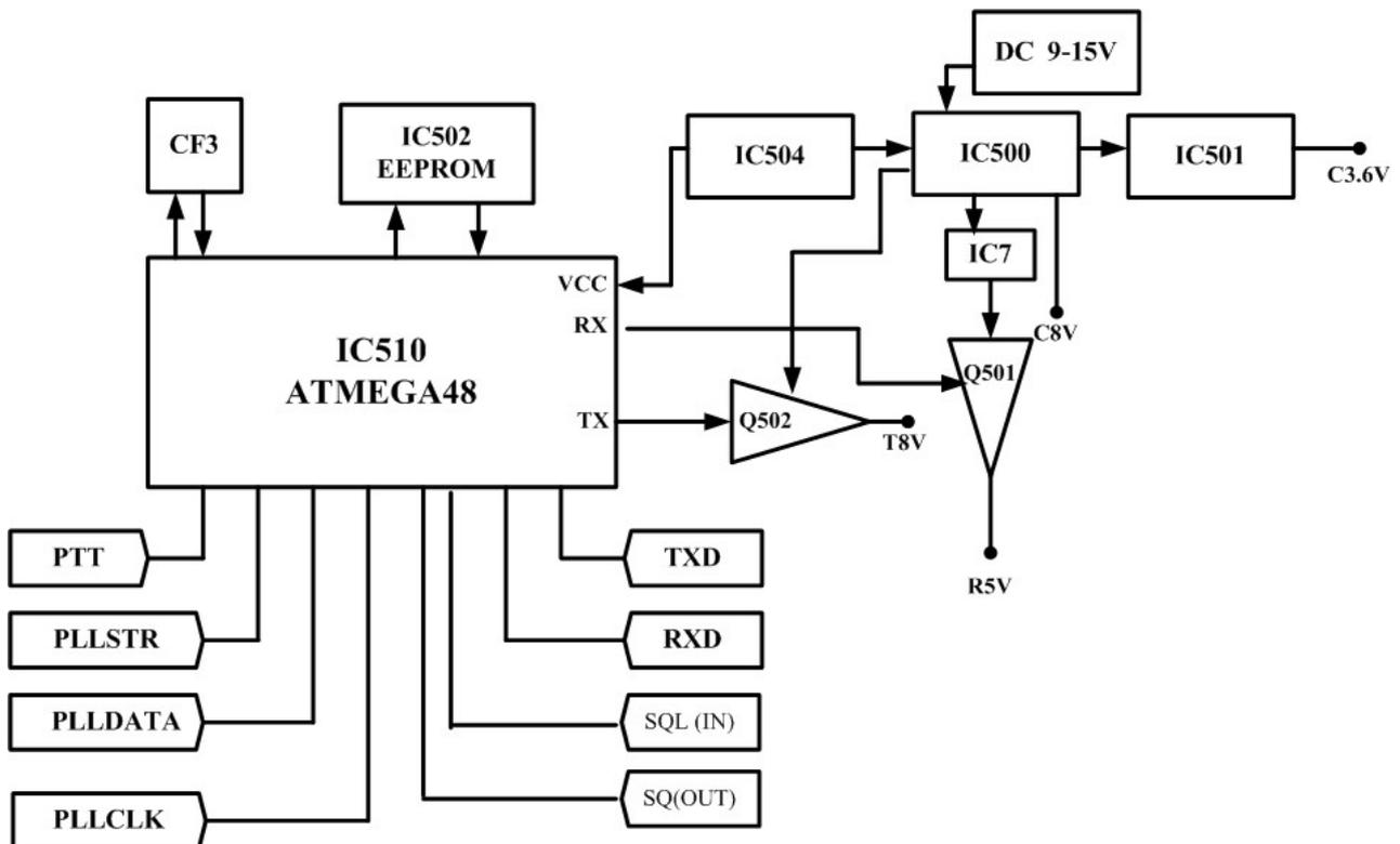
From Block Diagram above: The DC power was regulated to 8 volt by IC500 ,and supplied to the RF part. IC504 convert 8 volt to 5volt and supply to IC510. Q500 is RX power supply switch, Q502 is TX power supply switch. IC501 supply 3.6V to PLL IC. Channels can be selected by the switch (CF3). IC510 controls digital frequency synthesize by PLL STR ,PLL DATA and PLL CCK.
