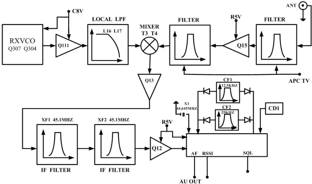
The receiver utilizes double conversion superheterodyne (UHF)/(VHF).
