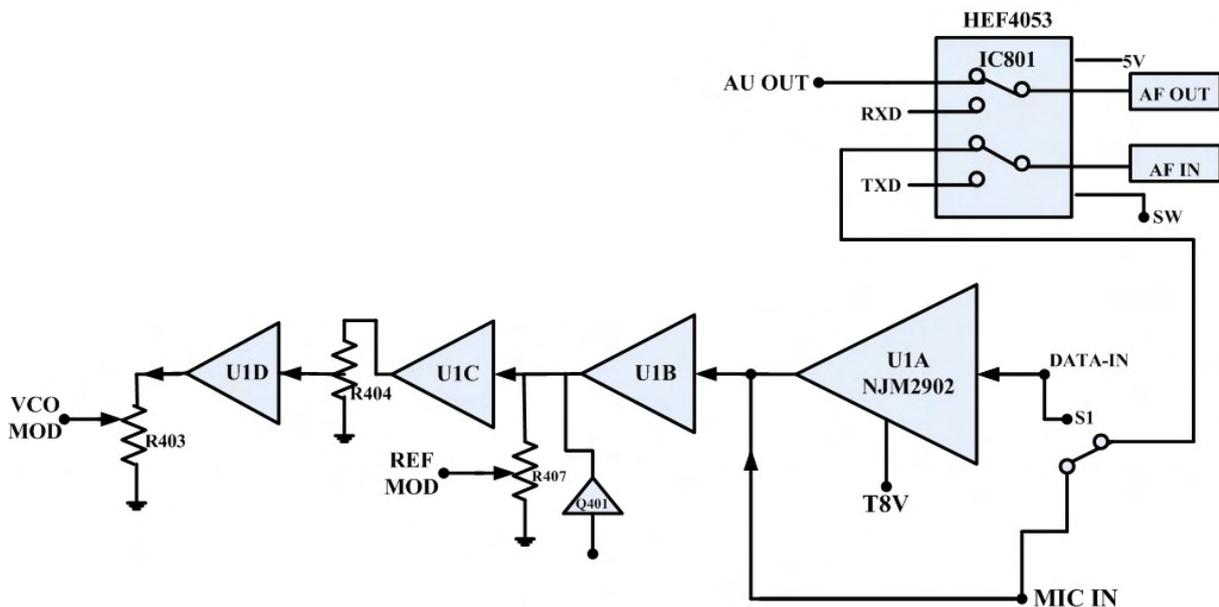
From the above Block Diagram : IC801 is audio/Data and UART signal switch. When the SW pin is high ,audio/data signal can go through IC801. S1 is a switch between audio and data input, when transmit audio, MIC IN port is shorted, when transmit data, DATA IN port is shorted. As it was data signal it will pass through DATA-IN port and amplified by U1A, then it was coupling by C431 and pass to U1B for amplify again;as it was audio signal it will pass
