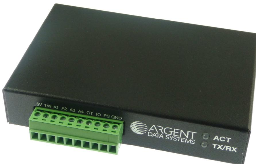
The front panel has two bi-color indicator LEDs, marked ACT (activity) and TX/RX (transmit/receive). The removable 10-pin terminal block is an accessory port that provides a Dallas 1-wire data bus, 5 volt power, four 0 to 20v analog
