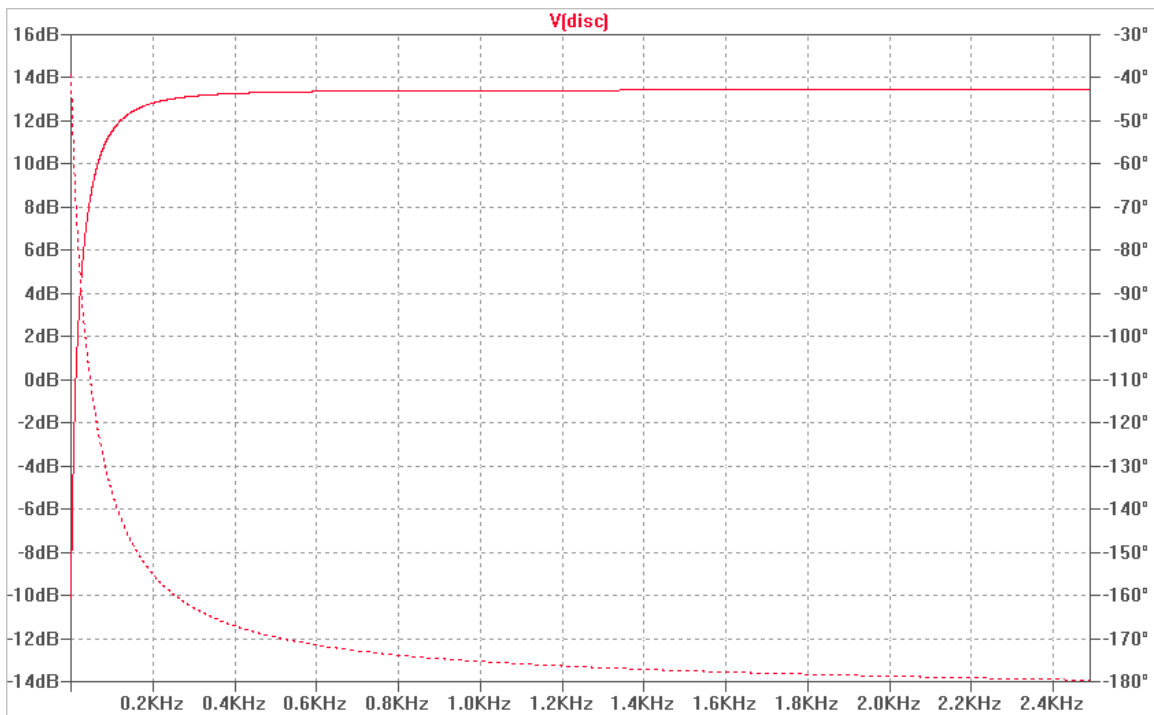
RX filter response, EQ jumper installed
