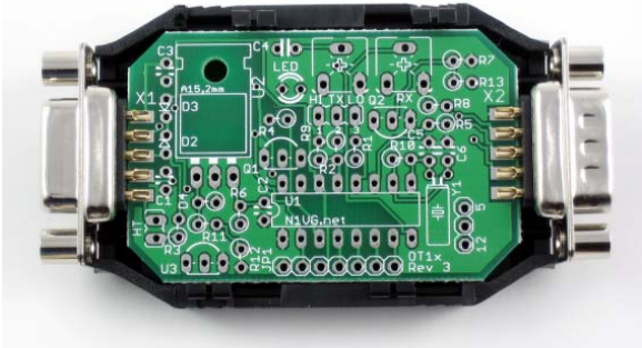
Board aligned in the lower half of the case, ready to solder the connectors in place.
