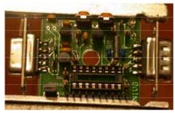
5. Finished project. In this case R3 has been left out as this unit will be used with a mobile rig
