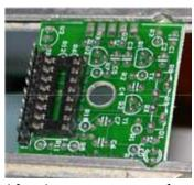
2. Start with microprocessor socket and 10-pin header
